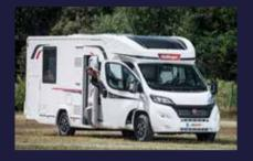
As of this year, ALTHEORA manufactures the front roof of the CHALLENGER & CHAUSSON brand's emblematic motorhome. Using composites improves the quality of the product and makes it easier to install.
